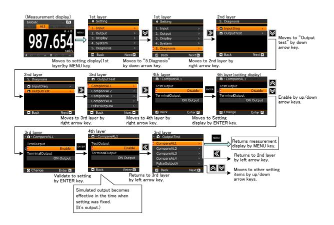
\*To stop simulated output, set "simulated output setting" to "Disable" or turn the power once.
