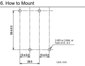
It's possible to install close adherence, but recommended so that 6.5 mm-more than 7 mm may be opened for thermal radiation.
