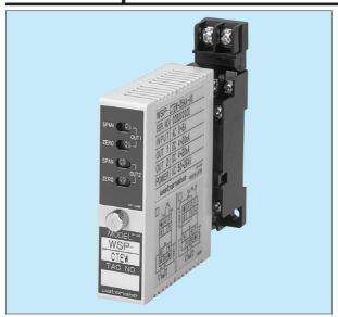
This compact plug-in signal converter with two insulated outputs converts the secondary outputs of CTs in power substations, motor circuits, etc. into DC signals. Since Type CTEW adopts the true root-mean-square value operation system, it ensures particularly high reliability against distorted waves.
