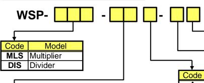
ŧ Code Input Input Resistance **10** 0 to 10mVdc 1MΩ 11 0 to 100mVdc 1MΩ **12** 0 to 1Vdc 1MΩ 13 0 to 5Vdc 1MΩ 1MΩ 14 1 to 5Vdc **15** 0 to 10Vdc 1MΩ 0 to 50mVdc 16 1MΩ 17 0 to 60mVdc 1MΩ 0 to 1mAdc 50Ω 32 **33** 0 to 10mAdc 50Ω **34** 0 to 16mAdc 50Ω 50Ω **35** 0 to 20mAdc 50Ω **36** 4 to 20mAdc Contact us for other than the above Full Scale Range: 99
