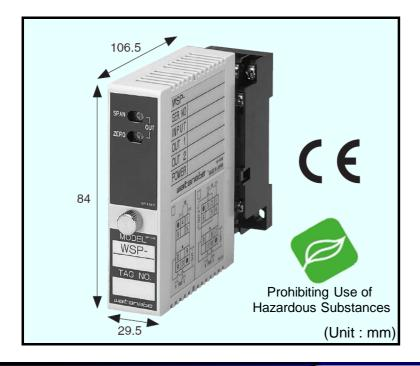
This compact plug-in signal converter (distributor) with output supplies 24Vdc to the 2-wire transmitter through signal lines and converts the signals (4 to 20 mAdc) to the DC voltage or current output.
