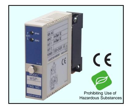
This compact plug-in, high-speed response type converter (isolator) provides signal output which is mutually isolated between input, output and power-supply. It amplifies and converts various kinds of signal with isolation to use in the integrated instrumental control system. It is highly effective as noise countermeasures.
