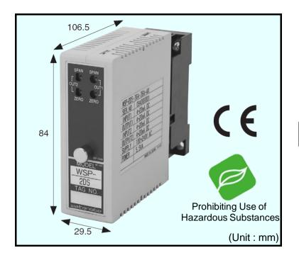
This compact plug-in converter (isolator) has 2 separate input / output circuit. This converter accepts a 2 channel DC voltage or current input and provides optically isolated DC voltage or current output. It amplifies and converts the selected DC input to the selected DC output. And also provides isolation of up to 2000V between the signal input, outputs, and power supply.
