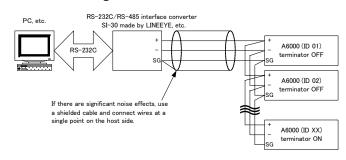
If cascade wiring is carried out with a RS-485 connection, use a commercially available Y-type split connector or the like.
