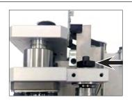
9 Move the R axis ball spline down and then remove the old timing belt.
