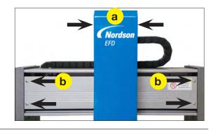
2 Move the Z axis module to the left side of the X axis.
