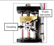
20 Release the four (4) screws that fasten the R axis motor to the R axis module.
