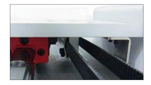
9 To add tension to the belt, tighten the timing belt adjusting kit base screw that sits in the front opening of the robot where the control assembly was previously installed.
