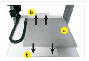
2 Move the fixture plate to the very back of the robot.
