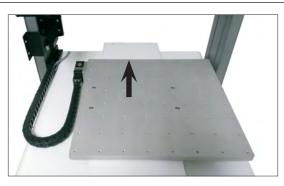
3 Carefully pull the Y axis cover away from the robot.
