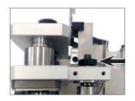
11 With the sawtooth sides of the new timing belt facing one another, loop the belt around the R axis idler and timing pulleys.
