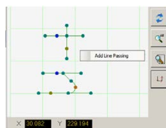
Right-click to stitch a Line Passing point onto an existing point
