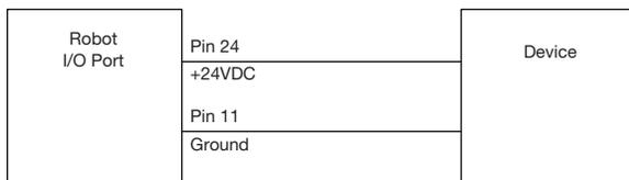
Courtesy +24 VDC output is rated at 3.0 Amp.
