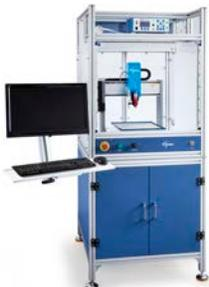
Nordson EFD guarded safety enclosures integrate seamlessly with our complete line of automated dispensing systems. Featuring external dispensing controls, a safety light curtain, and an internal electrical control box and wireways for faster, safer setup, these CE-compliant enclosures also fully comply with EU Machinery Directive 2006/42/EC.
