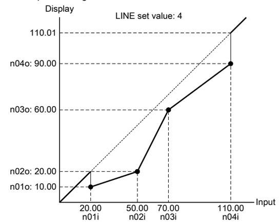
N.B.) If the linearize point changes do not fulfill the setting conditions, linearize correction may not execute correctly. Please ensure that linearize input and output values fulfill the setting conditions before commencing measurement.
