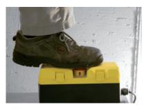
the control station. The installed devices will remain unaffected, thanks to the shape of the protection, which allows the pressure exerted to be dispersed onto the robust structure of the control station.
